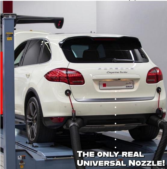
The innovative exhaust nozzle TMS 225 was developed according to the "one fits all" concept and fits on all exhaust pipe shapes without any restrictions.
